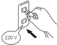
Do not use a power source exceeding the equipment's specified value. Use only 220-240V AC, 230V AC power or 24V AC adaptor if necessary!
