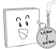
**Do not use this water softener under high water pressure conditions!**
