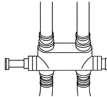
**Diagram 5:** Example of a Commercially Available Bypass Valve
