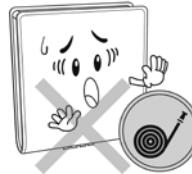
Unit should be installed and connected to the water mains by new hose-set that was included in the product package. Old hose-sets should not be reused with the unit.
