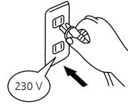
Do not use a power source exceeding the equipment's specified value. Use only 230V AC power!
