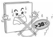
Water purifier inlet water temperature should not exceed 38°C!
